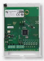
transceiver or repeater to expand lares 4.0 control panel
