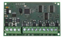
**auxi-A** is an expansion module that gives the opportunity to increase the number of inputs or outputs up to 5 on the lares 4.0 control panels.
