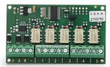
auxi relay has 5 relay outputs (1A) which may be used for manage all kind of loads in lares 4.0 Control Panel series. auxi relay is programmed directly from lares 4.0 Control Panel.
