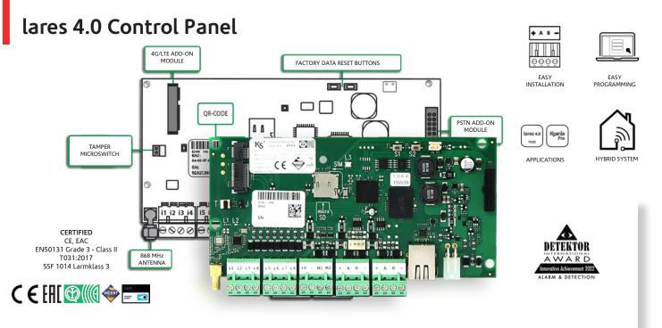
The core of the whole system is inside the hybrid IoT Platform **lares 4.0**. It's a hybrid because it includes both wired and wireless systems and has an equal number of inputs and outputs for the management of lights, HVAC, irrigation, shutters and any other kind of automation or household appliance, involving both Security and Home Automation.
