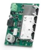
switch 4.0 is a 10/100Mbit Ethernet network switch, designed to connect the Control Panels Sistem lares 4.0 with our IP modules (ergo-T/ergo-T pro, gemino IoT, porta etc).
